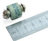
Note3. If K15Y-1 capacitor used as shown on a photo below, no terminals required as those capacitors can be soldered directly to the board.
